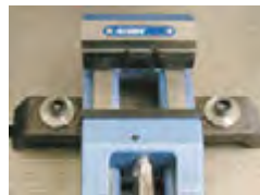
Clamping with clamping brackets
