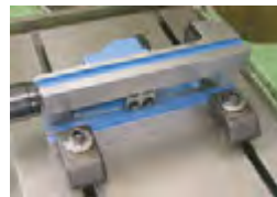
Clamping with clamping brackets, laterally
