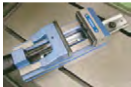
Clamping with guide rail
