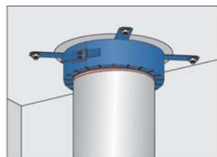
Solid ceiling fixed with dowels
