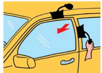
2a: The Winbags can be pumped up carefully until there is enough space to slide the locking system in.
