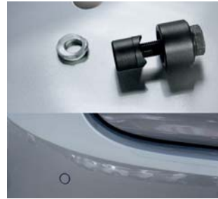
3. Precision-fit punched hole for parking sensor
