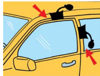
1a: One or two Winbags are inserted between the car door and the frame. The Winbags will be easier to position if they are first sprayed with FÖRCH silicone spray.
