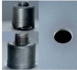
2. Apply the punch on painted side and punch out by screwing down
