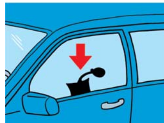
1b: Place one or two Winbags between the window pane and the rubber strip on the car. Slide the Winbag in place as shown on the illustration.
