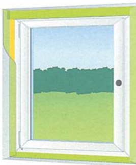
Picture 3: Turn over the window tape and adhere the self-adhesive tape along the window frame.
